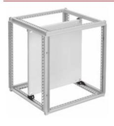
ProLine Mounting Plates are designed to provide maximum panel depth, panel size and ease of installation. Mounting Plates slide into the frame on nylon glide blocks, which support the entire weight of the mounting plate.
