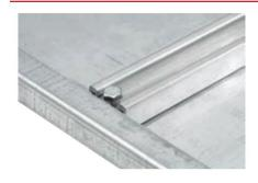
Panel Support Braces give additional support to single- and double-bay panels in heavy loading applications and minimize the vibration created by components mounted on the panel. Braces can be installed on existing systems without removing the panel. Panel support braces are furnished in pairs. Braces are unpainted galvanized steel.
