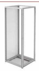
Side mount mounting-plates can be installed on the interior sides of frames. The panel and all the hardware needed to attach the mounting plates to a frame are included. Hardware is plated. Panels are 2,5 mm galvanized steel.
