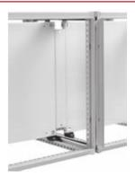
Provides a continuous panel surface in multiple-bay enclosures. The joining mounting plate is inserted between mounting plate of equal height. It can be installed from front or rear. Holes for grounding and mounting hardware are provided. Conductive mounting plates are unpainted galvanized steel.
